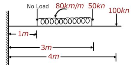
Draw shear force and bending moment diagram for the cantilever shown.
